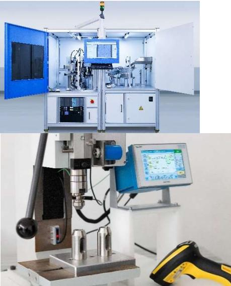
The KVC 821 optical inspection system from Kistler performs automated quality assurance at the end of the production line.
