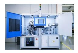
The KVC 821 optical quality inspection system for injection molding provides accurate 100% inspection of plastic parts using variable camera systems and Albased anomaly detection.
