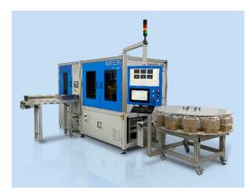
The Automated Vision Inspection system achieves, depending on the configuration, cycle times of two seconds from the moment the test piece is picked up to the OK/NOK decision and the corresponding sorting.
