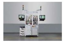
The new Inline Vision & Weld quality assurance system combines optical quality inspection and laser welding technology for seamless punching strips with exclusively inspected OK parts.
