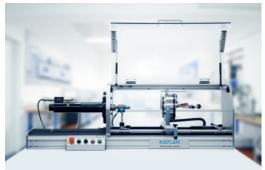
Analysis system from Kistler for determining friction coefficients on bolted joints
