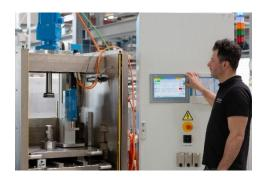
Kistler now offers traceable on-site and in-situ calibrations for force measuring chains and joining systems up to 300 kN.
