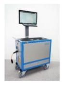
Torque tools such as cordless, rotary, and impulse screwdrivers can be tested in a standard-compliant and mobile manner with the cerTEST inspection system.
