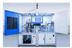
With the new multicapture device, the KVC 821 optical quality inspection system from Kistler detects the smallest defects on the surface of the test parts, even at high cycle times.
