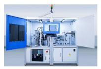
Automatic optical quality testing systems from Kistler check the dimensions, colors and surface characteristics of injection-molded products.
