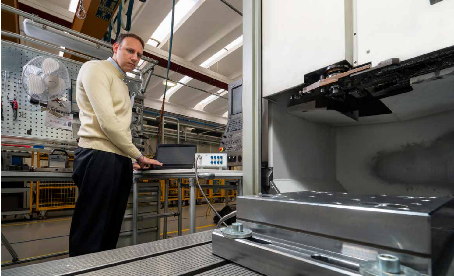
Electrospindle development at HSD Mechatronics: Manuel Camperchioli regularly works with the 9255C dynamometer from Kistler to analyze machining dynamics and to foster innovation.
