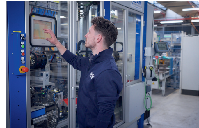
Product quality and maximum repeatability are no problem thanks to the maXYmos NC process monitoring system. Daniel Egri from TEAM Automation Berlin takes a look at the force-displacement measurements.
