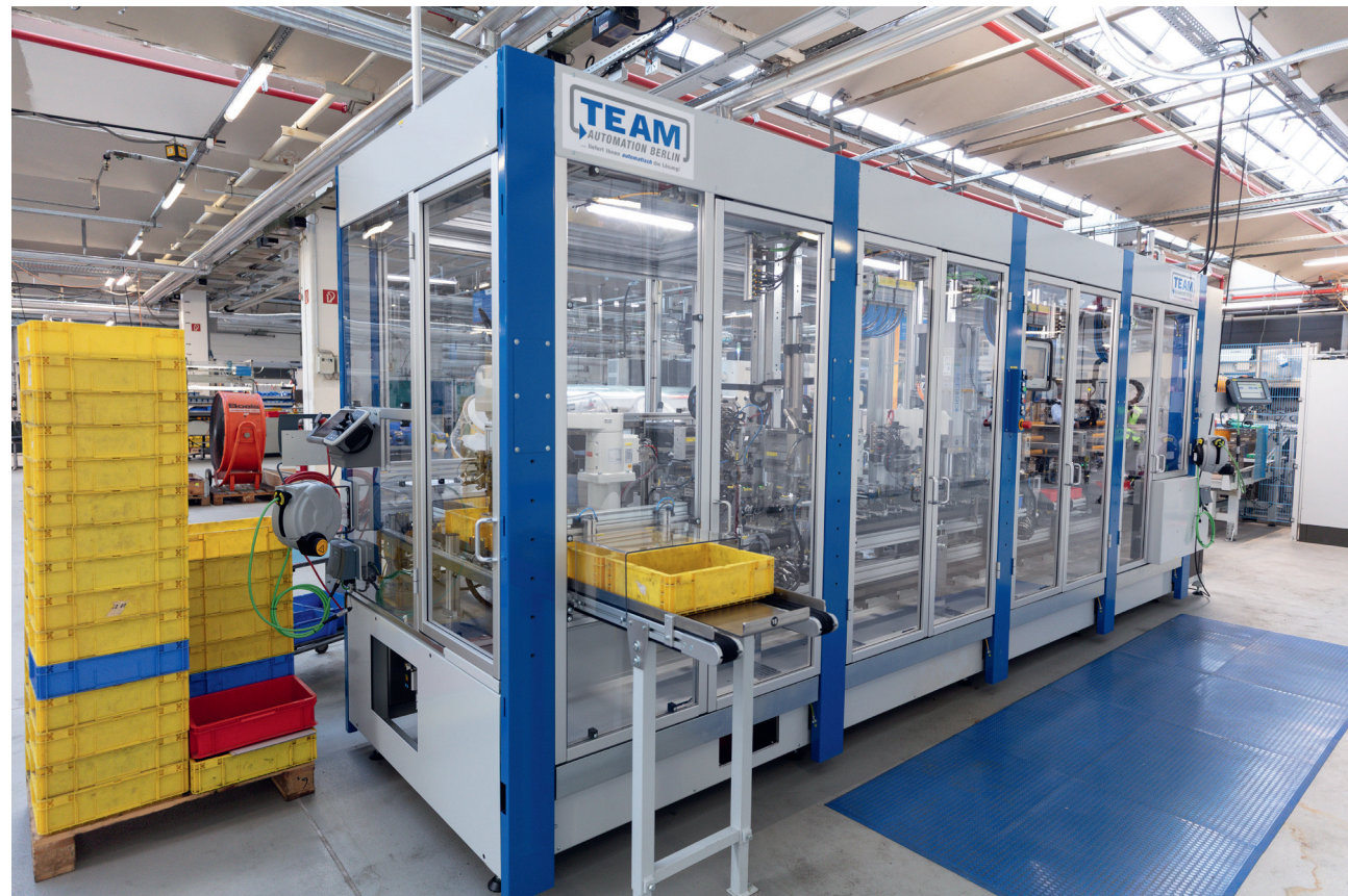
Fully automated assembly line for lubricant distributors featuring a wide range of variants, precise press-fitting and assembly technology, and short cycle times – supported by Kistler's servo press NCFE and the process monitoring system maXYmos NC.
