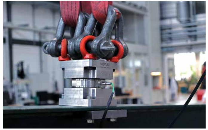
Measurement technology from Kistler in detail: The piezoelectric force sensor 9377D up to 150 kN is installed between the load harness and crane suspension, and measures the load applied to the wing dynamically and with a high degree of precision.
