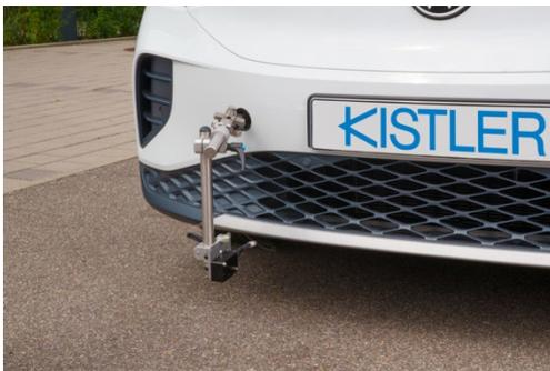
Correvit KiMotion Racing's optical sensor head can be installed not only on racecars for vehicle dynamics measurements, but also on standard road vehicles. Installation types: External installation on the vehicle (as shown), direct installation on the wheel, on the vehicle chassis or behind cladding – as standard in motorsport. Kistler also offers the corresponding accessories to ensure optimal installation on the vehicle.
