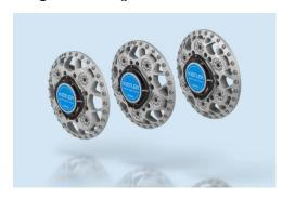
The 6-component wheel force transducers in the RoaDyn Integra series (4, 5, 6) capture wheel forces (from 25 to 65 kN) and moments (from 4 to 12 kNm). They are used for vehicle development and testing, on test tracks as well as test stands. The wheel force transducers are positioned on the relevant rim and mounted on the vehicle with the help of the matching hub adapter.
