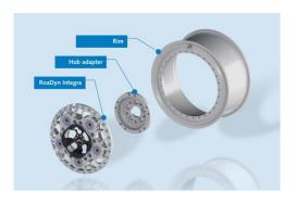
The structure of the RoaDyn Integra wheel force transducers comprises the Integra sensor assembly, the data transmission (standard: outboard transmission), rim and hub adapter. The hub adapter and rim are exchangeable, so maximum flexibility is ensured.
