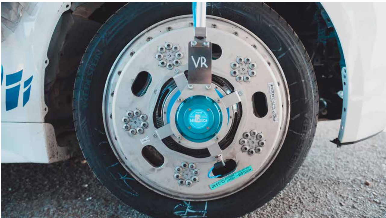
Designed for performance, Kistler's RoaDyn wheel force transducer (WFT) measures forces and moments on the wheels during dynamic maneuvers, providing precise data essential for optimizing vehicle performance and tire behavior under extreme conditions.
