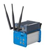
The KiRoad Wireless onboard electronics from Kistler receives the signals from wheel torque transducers such as the new RoaDyn P109 and offers various interfaces such as CAN, DTI and Ethernet.
