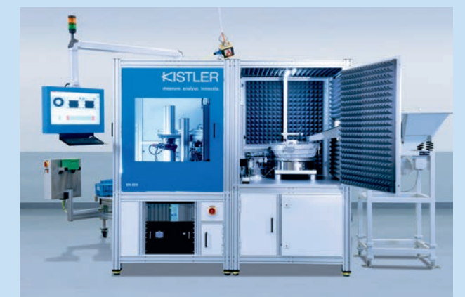
Variant of the KVC 821 automatic testing and sorting system with continuous feed, but test objects are clocked to pass through the individual test stations on the rotary plate.
