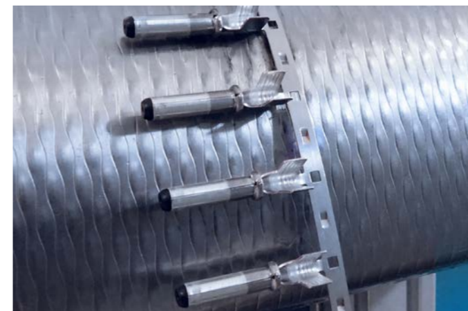
The quality of the continuously produced high-voltage connector from KRAMSKI – the black plastic cap is on the left side of the connector in this photo – is guaranteed with the help of process monitoring and further test systems from Kistler.
