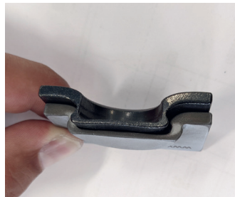
Clinching is a joining technology that permanently joins two different layers of material (such as two metal sheets or plates) by means of a force-fit and form-fit connection.
