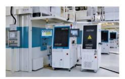
With a laser marking system from Kistler such as the KLM 621 shown here, markings can be applied to as many as 2,500 parts per minute.
