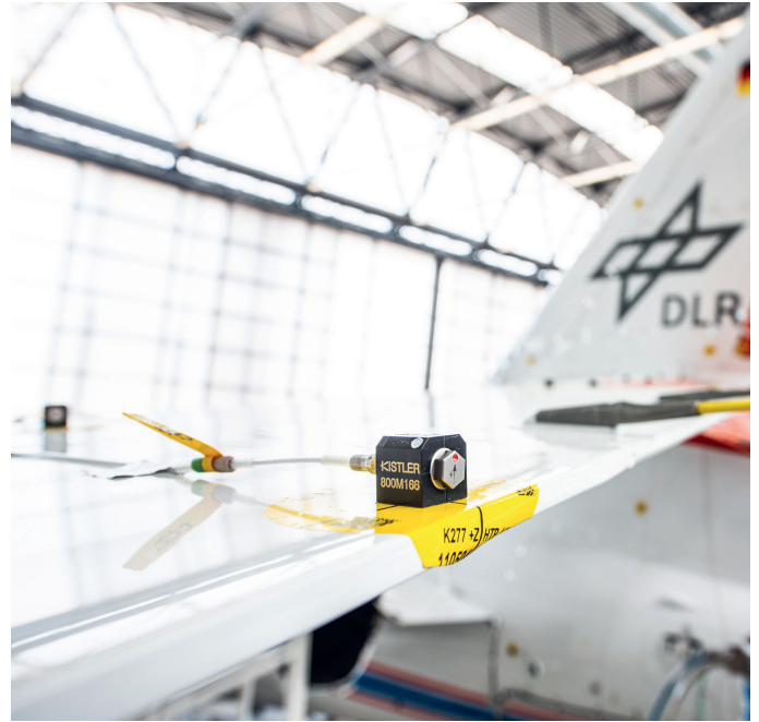
For ground vibration testing on the ISTAR, the DLR uses over 200 IEPE accelerometers from Kistler. They feature exceptional temperature stability and movable alignment. © DLR
