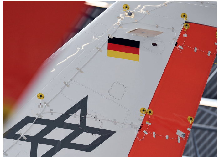
For the ground vibration test, accelerometers from Kistler are positioned on various parts of the aircraft – the tail unit of the new ISTAR in this case. © DLR
