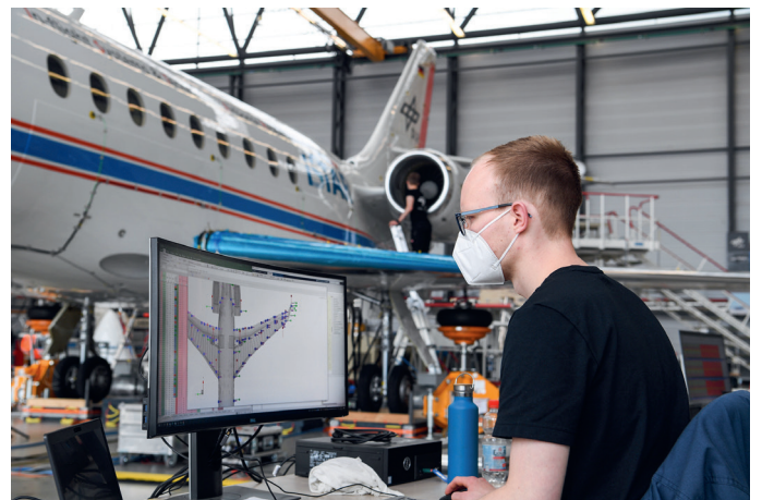
The DLR's ISTAR research aircraft was equipped with over 250 accelerometers from Kistler for vibration tests on the ground and in the air. © DLR
