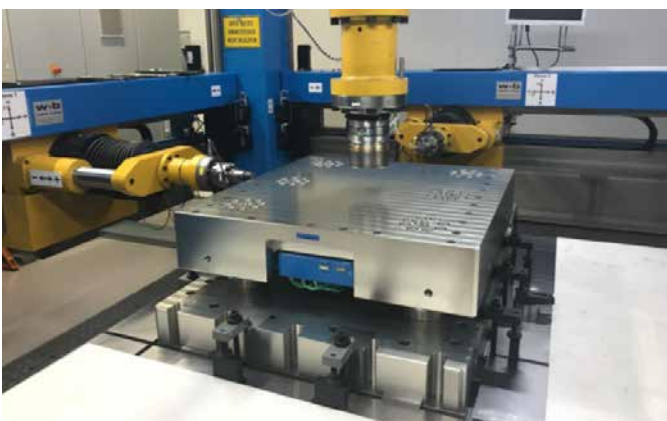
Fig. 20: 3-component force link 9397C (-200kN to 450kN range) Fx, Fy up to ±100 kN, Fz: -200 ... 450 kN
