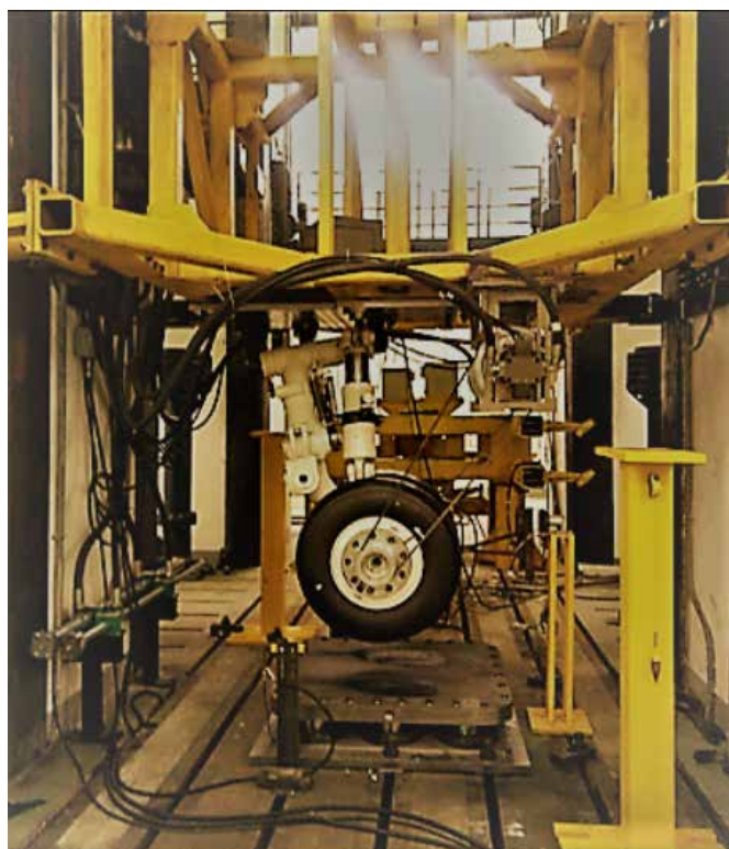
Fig. 22: Drop test stand and landing gear under test using Z21594 dynamometer
