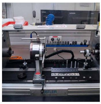
The laboratory test stand for precise determination of friction coefficients: the ANALYSE system from Kistler features a modular structure, and it can be equipped with multiple drives and a vibration test stand.
