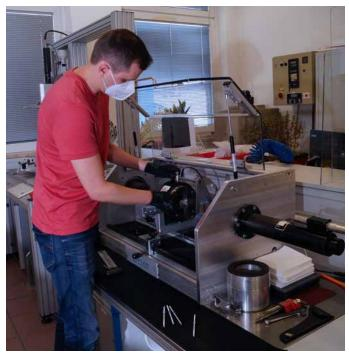
An ANALYSE system from Kistler – operated here by Quality Engineer Eduard Buch – is used almost every day to determine friction coefficients in the laboratory at Dörken's headquarters.
