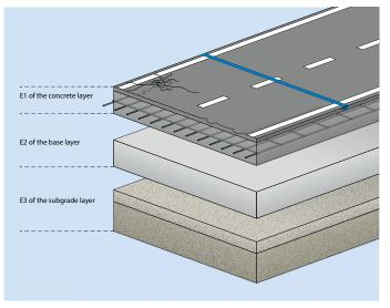
Road structure and quality have a significant influence on the accuracy of Weigh In Motion (WIM) systems: advanced methods integrated in a new service from Kistler ensure optimum WIM performance.
