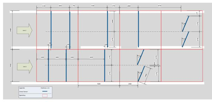
Recommended sensor layouts for Weigh In Motion on lanes 1 and 2 of highway D2 in the Czech Republic (km 8.3, Brno-bound) – generated by the new Structural Road Analysis service from Kistler.
