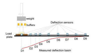
An analysis based on measurements with a Falling Weight Deflectometer (FWD) – part of the SRA service from Kistler – delivers key data on road pavement structure and the quality of the different layers.
