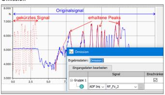
Convenient shortening of any number of measurement signals simultaneously, taking the damage and extremal values into consideration, as preparation for a test run on multi-axial test stands:
