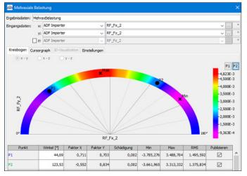
Preparation of single-axial trials in which load signals are vectorially combined in two or three directions and assessed using the damage:
