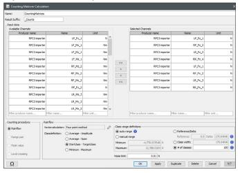
The Rainflow analysis determines a two-dimensional distribution. It is mainly used to analyze life expectancy. The results are output as a matrix.
