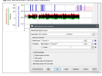
The calculation determines outlier values in a measuring signal and corrects them in a definable mode. Spike detection is easy to configure by defining a range of permitted values.
