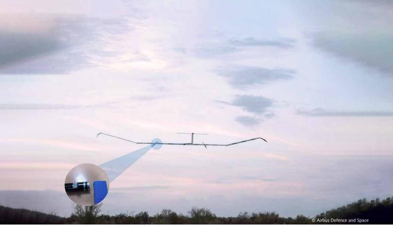
A cryogenic K-Shear IEPE accelerometer from Kistler is part of the flight test equipment of Airbus' HAPS Zephyr for persistent operation in the stratosphere.
