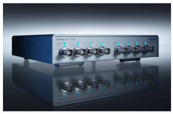
Data acquisition for ground and flight testing for Airbus Zephyr was done using the laboratory charge amplifier LabAmp 5165A from Kistler with his flexible user interface and daisy-chaining capabilities.
