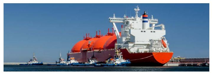
LNG (liquefied natural gas) tankers carry the liquefied natural gas around the world in special containers.
