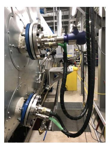
Custom cable solution from Kistler for pressure sensors inside the autoclave (left) of The Atmosphere sloshing test facility at the MARIN research institute in Wageningen (Netherlands)
