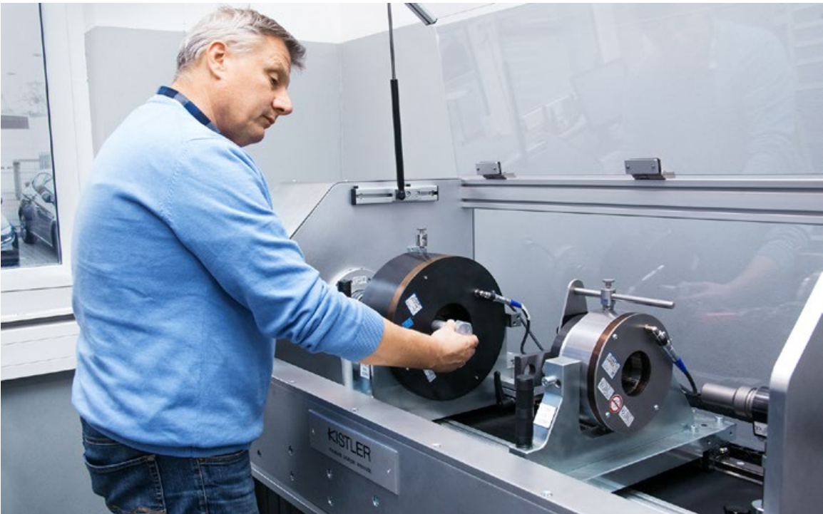
Our ANALYSE system ensures reliable design and accurate testing of threaded joints – no matter how small or large they are.
