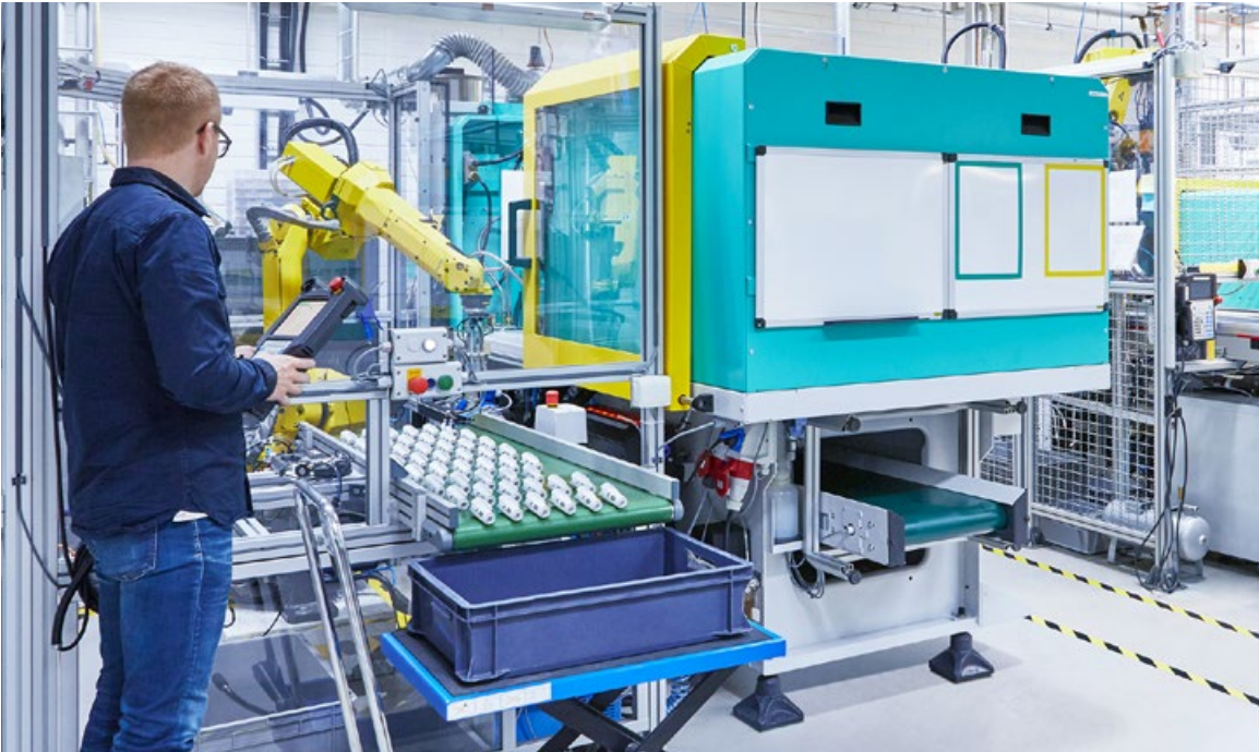
Sensor technology installed in the mold is the basis for capturing all material-related and part-specific attributes – adding up to the part's fingerprint.
