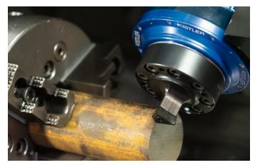
The 9171A 4-component rotating cutting force dynamometer (RCD) was used to measure the cutting forces. Piezoelectric sensor technology gives the RCD a very high sampling rate coupled with sensitivity across an extremely wide force range.
