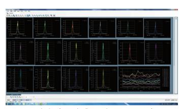
Measurement technology from Kistler allows simultaneous monitoring of injection and internal pressure on all 16 cylinders.
