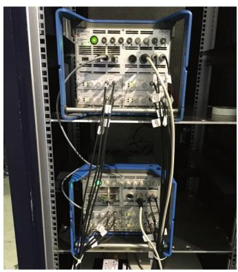
Using two cascading KiBoxes from Kistler, it was possible to monitor and optimize all 16 cylinders simultaneously.
