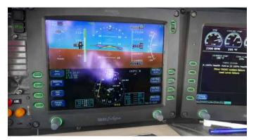
How do engine performance and flight characteristics change with altitude? A look at the instrument panel and the values measured by KiBox provides the answers.
