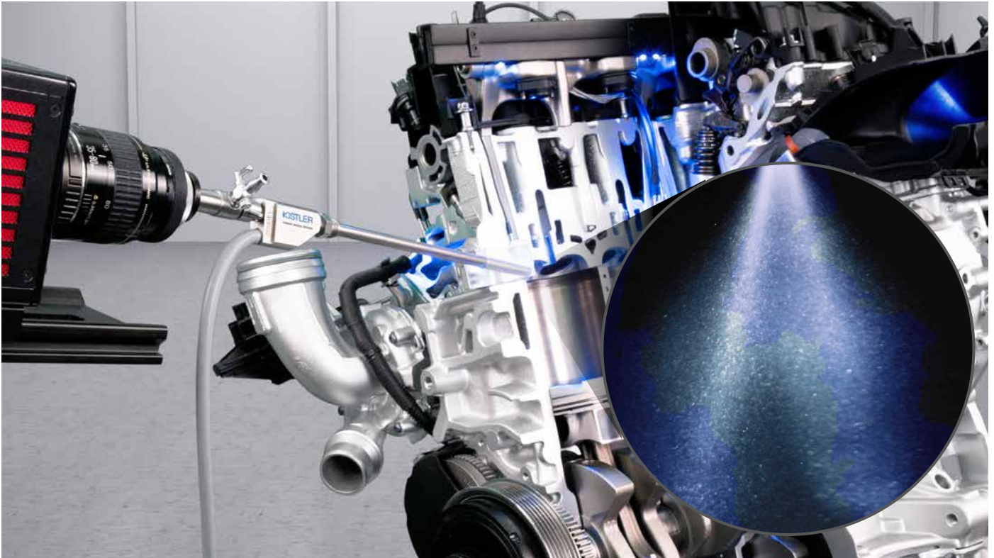
Schematic view of the high-speed camera system used to visualize the injection jet on a gasoline engine with direct injection
