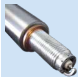
Serial spark plug with built-in optical windows
