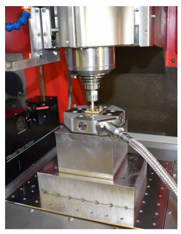
Thanks to MicroDyn from Kistler, the world's smallest dynamometer, the cutting forces on the tool can be measured precisely at speeds of up to 120 000 rpm.
