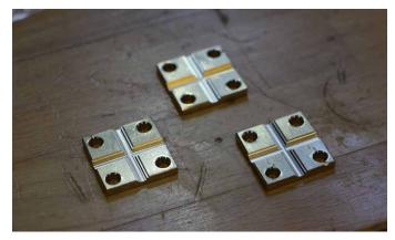
The brass plates undergo several machining processes with different apertures in order to acquire representative data.
