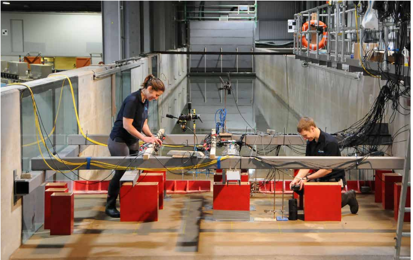
The English town of Wallingford is home to one of Europe's largest wave flumes, the Fast Flow Facility, where tsunamis can be simulated on a scale of 1:50. (Source: HR Wallingford)
