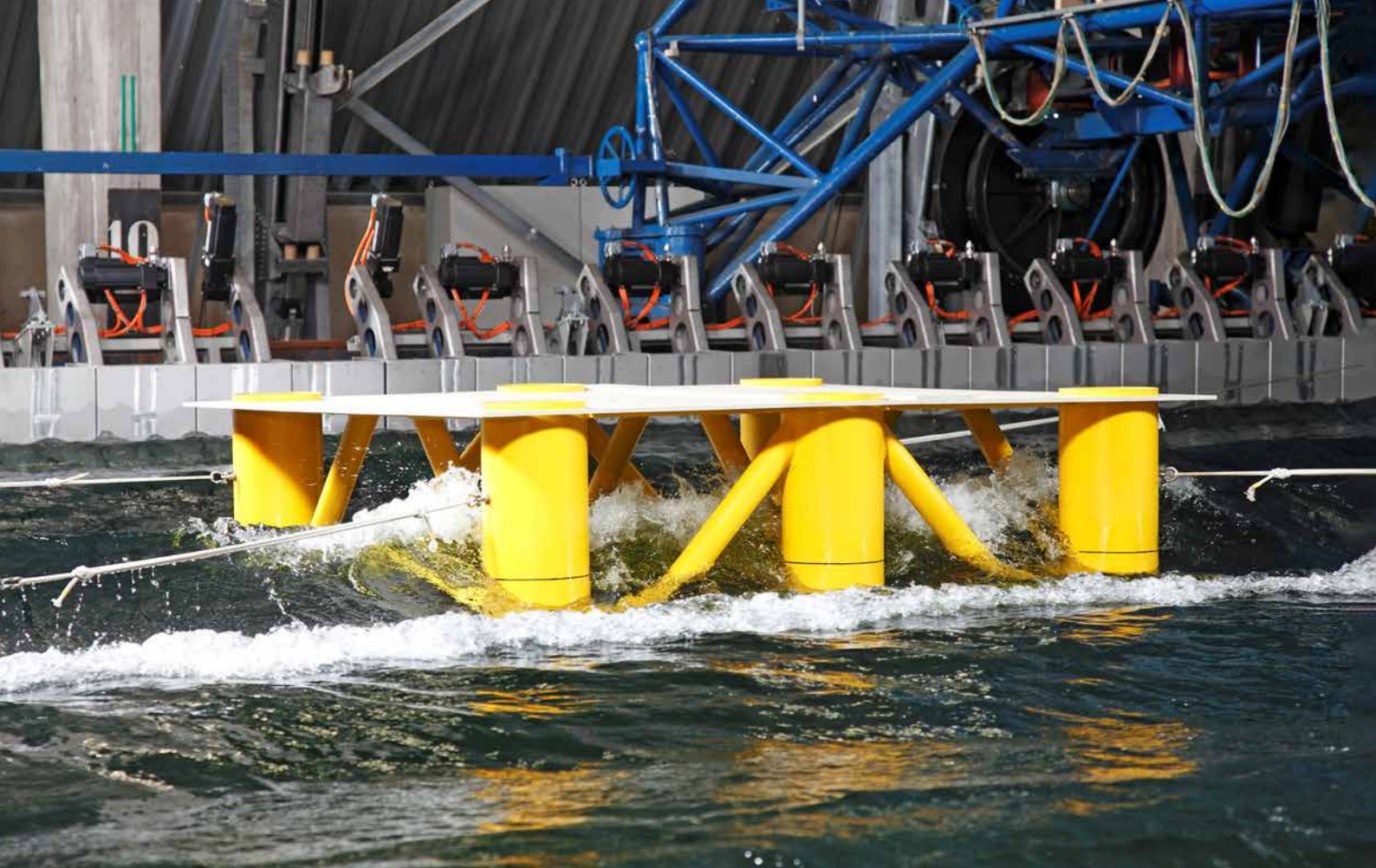
Slamming test in progress on an oil and gas platform model (Source: HSVA)
