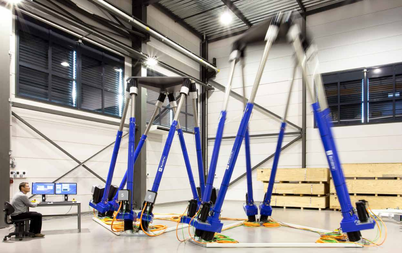
Sloshing simulation system using an LNG tank model mounted on top of a hexapod (Source: Symétrie)
