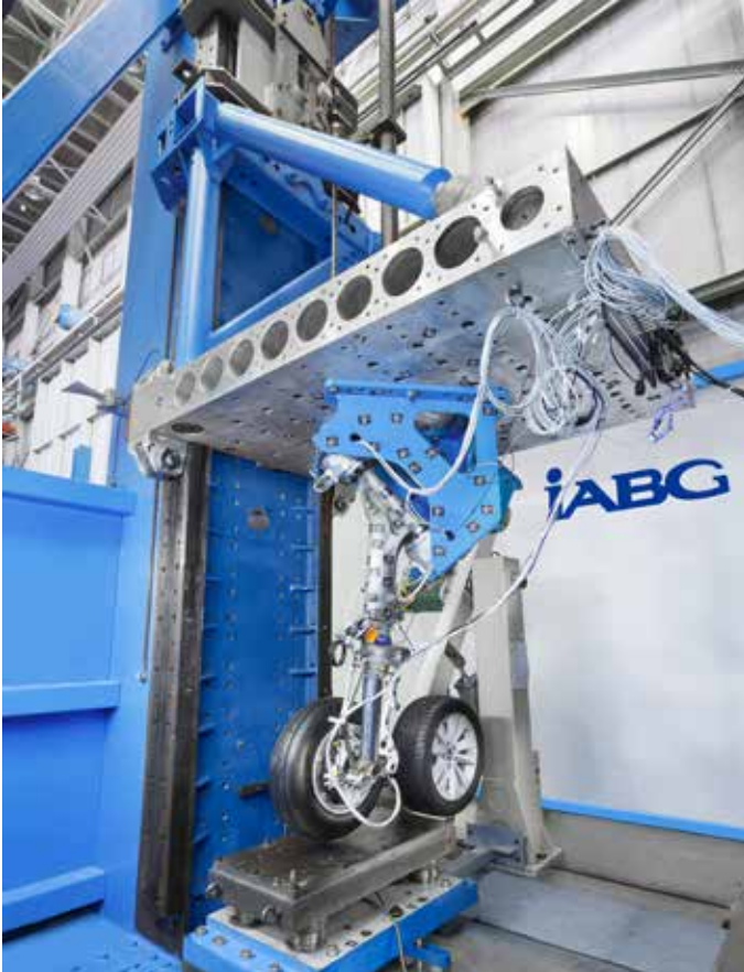
Functional test on landing gear (source: IABG).
