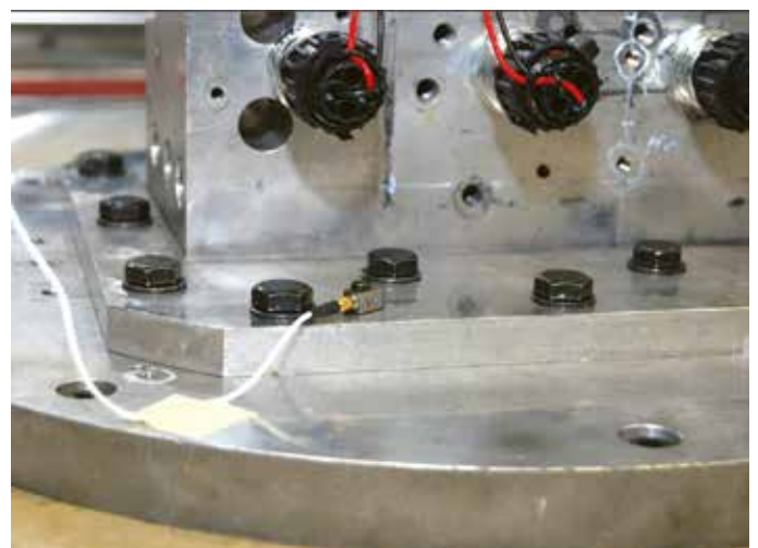
Type 8715B250 teardrop PiezoStar accelerometer mounted on an electrodynamic shaker in a thermal chamber for Highly Accelerated Life Testing (HALT).
