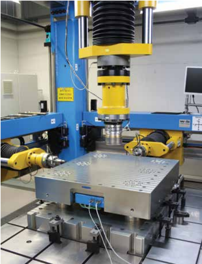
Calibration of a customized force dynamometer for the landing gear drop test on Kistler's special tri-dimensional calibration rig.
