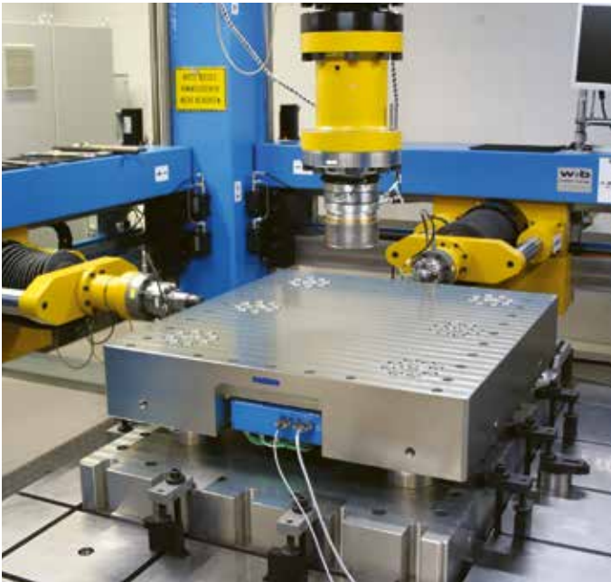
In-house calibration on Kistler's unique 3-component reference force press.
