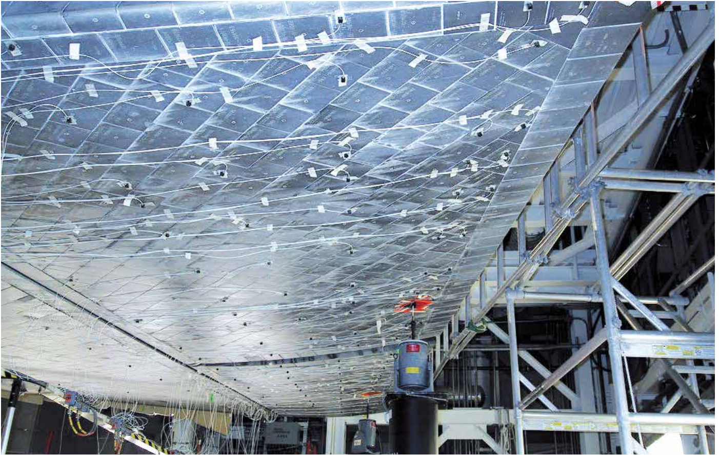
Ground vibration testing of a space shuttle.
