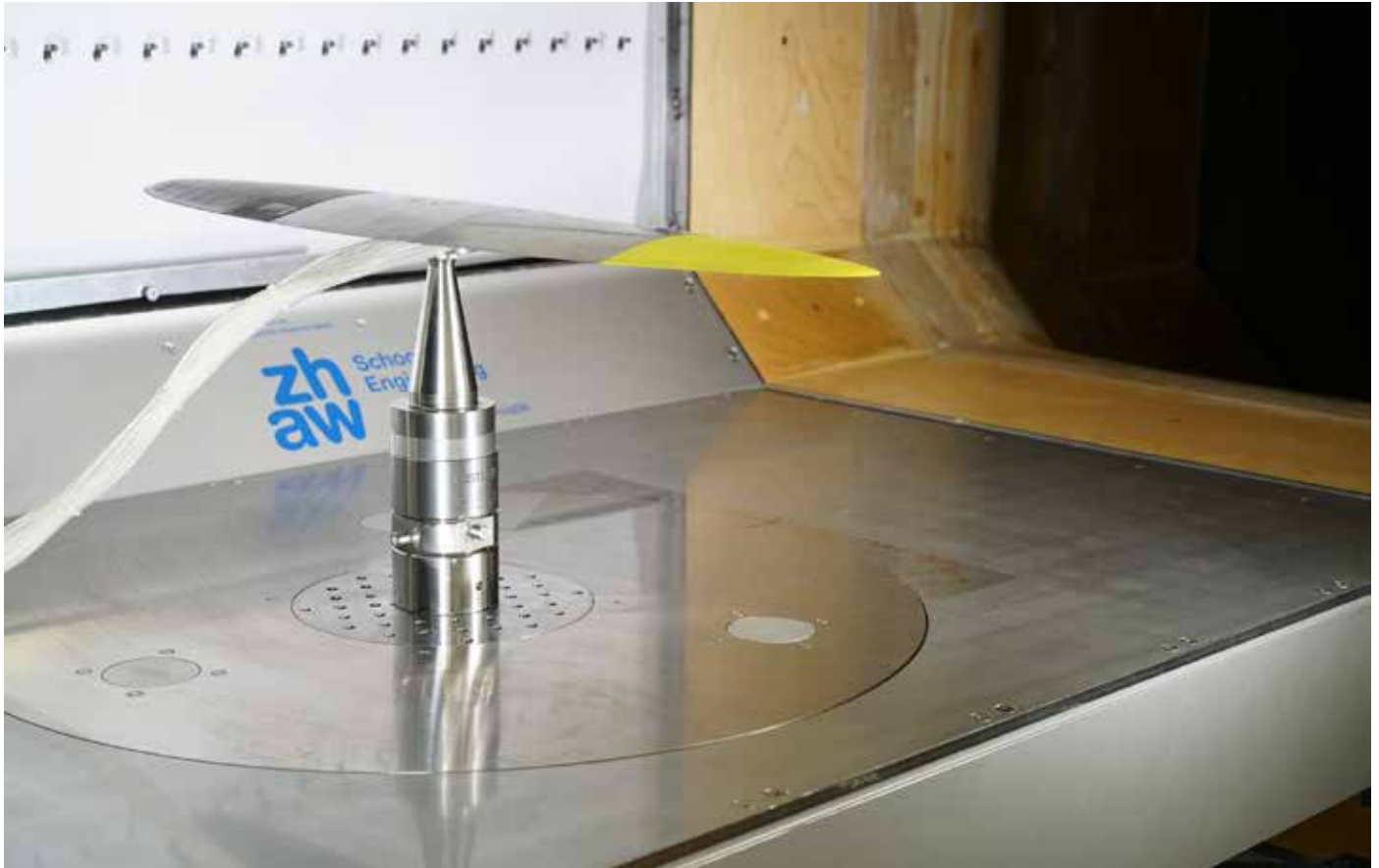
6-component force sensor Type 9306A in a wind tunnel application at Zurich University of Applied Sciences (ZHAW).
