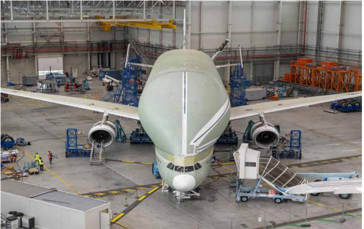
Prototype Airbus Beluga XL undergoes ground vibration testing (source: AIRBUS).
