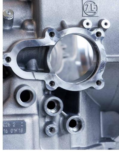
A component with different threaded joints
