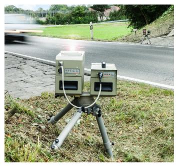
Monitoring of both directions of traffic with just one measuring system and two independent photo units.
