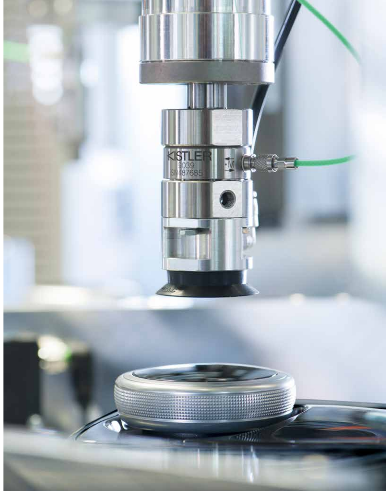
Haptic test using a Type 9039 piezoelectric torque sensor.
