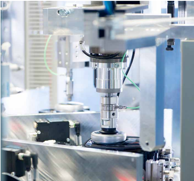
The torque sensor supplies data with a resolution of up to 0,1 Nmm at rotational speeds of as much as 180 degrees/s.
