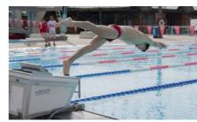
KiSwim system: Swimming system consisting of an instrumented starting block, turning plate and multiple above- and underwater cameras. Analyze your athlete's start and turn in our unique software with direct feedback.
