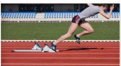
KiSprint system: Sprint system consisting of two instrumented starting blocks, a camera and a laser for speed measurement. KiSprint software provides insight into your sprinter's start.
