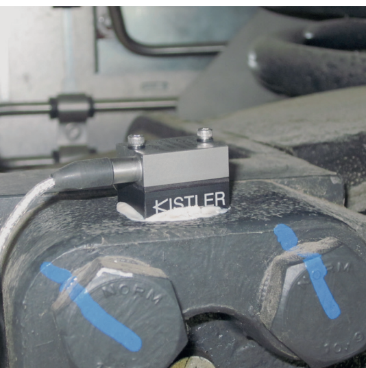
Usage of single axis Type 8316A for preventive maintenance on tramways
