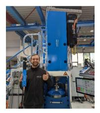
Steffen Schulz, Team Leader System Testing at Kistler in Lorch, holds the currently smallest NCFT joining module with telemetry and integrated force sensor in the plunger with a measuring range starting from 50 N and above. In the background the so far largest joining module NCFN with a measuring range of up to 700 kN is visible.
