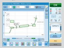
The XY maXYmos monitors oversee and evaluate the quality of a product or production step on the basis of two measured variables in relation to one another
