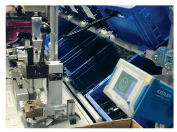
Ergonomically fitted manual workstation with integrated quality assurance
