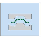
After curing, the mold is opened and the part can be demolded.
