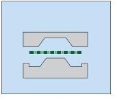
The impregnated fiber mats are placed into the mold. The time factor is relevant here because the reaction has already started. This is why robots are often used to perform this step.
