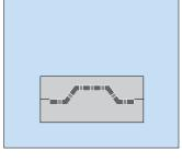
The binding powder added during stacking melts due to the heat impact and fixes the mats or fabrics in the correct shape.
