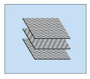
**1 Manufacturing the preform** Fiber mats or fabrics are stacked in a defined sequence and fiber orientation.
