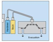
The cavity is evacuated after the mold is closed. This prevents air inclusions in the final product.
