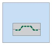
The resin continues to disperse as the mold closes, and the entire cavity is filled after complete closure.
