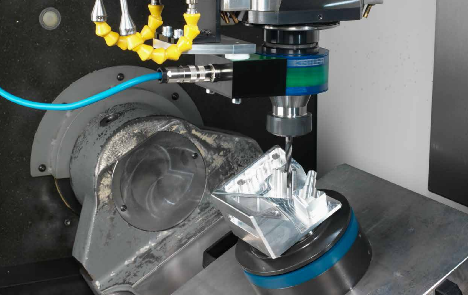
Drilling with a Type 9170A rotating dynamometer
