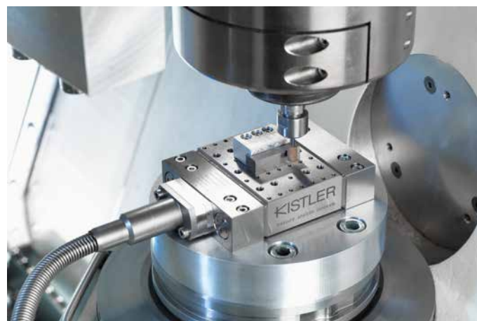
Grinding with a Type 9119AA2 dynamometer
