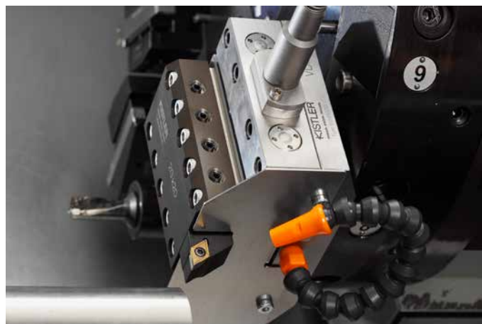
Turning with a Type 9129A dynamometer
