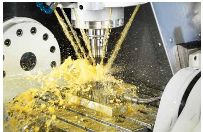
Milling with a Type 9129AA dynamometer
