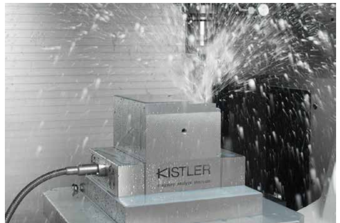
Milling with a Type 9139AA dynamometer
