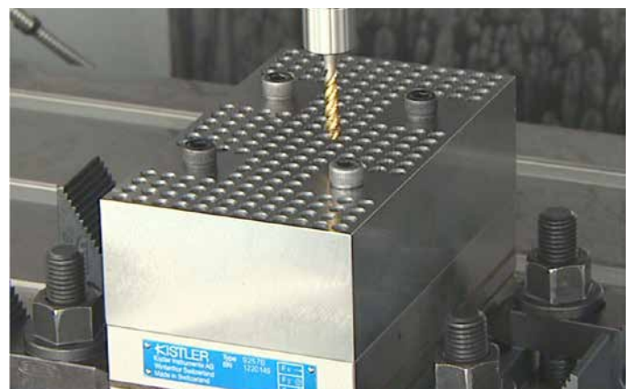
Screw tapping with a Type 9257B dynamometer
