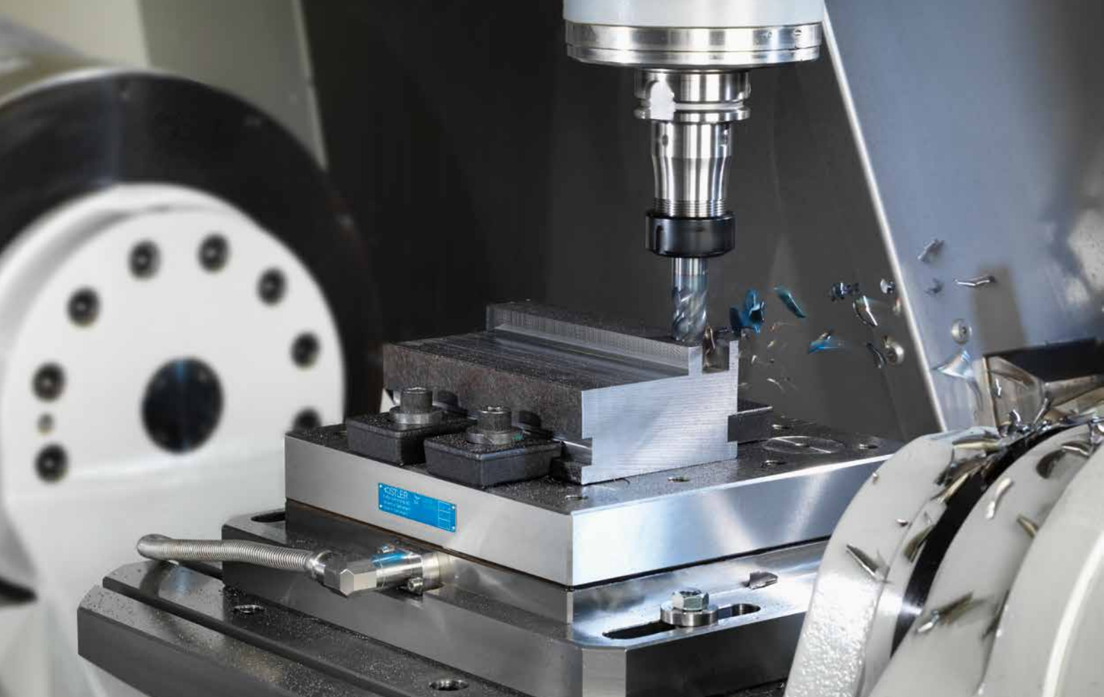
Milling high-alloy steel with a Type 9255C dynamometer
