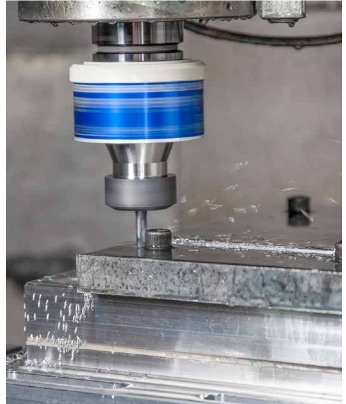
Rotating dynamometer in a milling application
