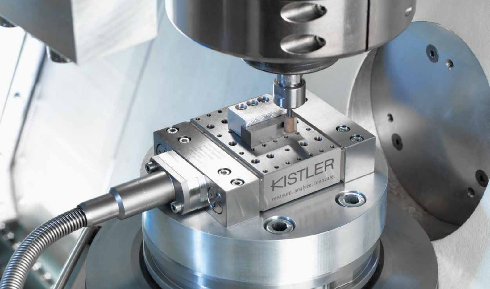
Grinding with a Type 9129AA dynamometer
