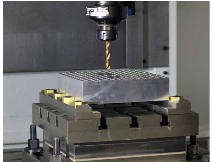
MITIS systems in operation: in this photograph, the workpiece is clamped onto a Kistler 9255C dynamometer
