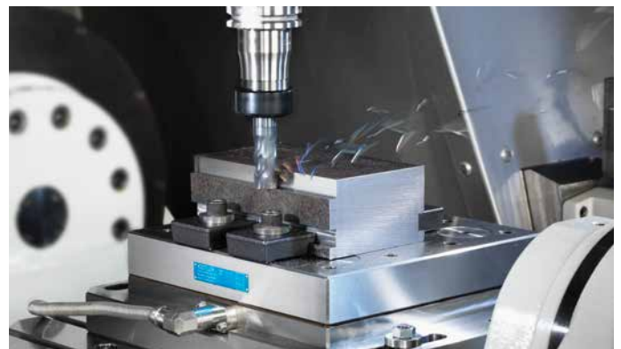
Milling with a Type 9255C dynamometer
