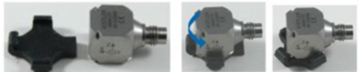
Figure 2: Type 8788A... with quick locking clip (+Z-Axis up)
